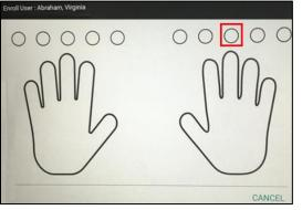
10. In the **Scan finger to enroll** prompt, the selected finger (In the following example, the middle finger of the right hand) is highlighted on the left side of the prompt. The employee follows the image on the right side of the prompt by placing the selected finger on the platen.
