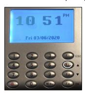
2. On the Enter Badge/ID prompt, you can place your enrolled finger on the platen or type the badge number using the keypad. When using the keypad, press the synchronization key to erase the number and re-enter it if necessary, press MENU to navigate among OK, Cancel and the edit field, then press F4 for OK to confirm your entry.
