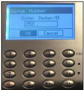
3. At the prompt, in this example DEPARTMENT, enter the workgroup identifier for the transfer. Press the synchronization key to erase the number and re-enter it. Use MENU to navigate among OK, Cancel and the edit field. Then press OK to confirm your entry.
