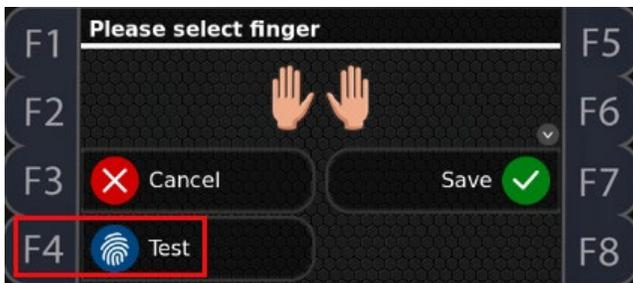
2. When the Verify... prompt is displayed, place the enrolled finger on the platen.
